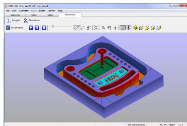
The FILOU-NC-Simulation supports three simultaneous axes.
