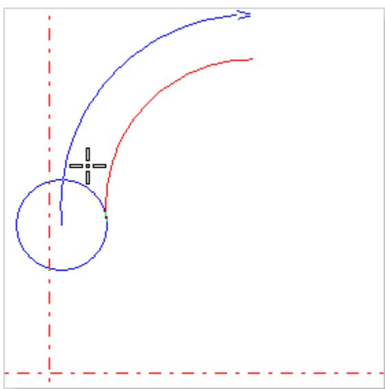
Right and left is referring to the milling direction which is defined by the starting point of the contour as already explained. Move the cursor over the geometry. FILOU-NC displays the current path correction. A click with the left mouse button confirms your selection.
