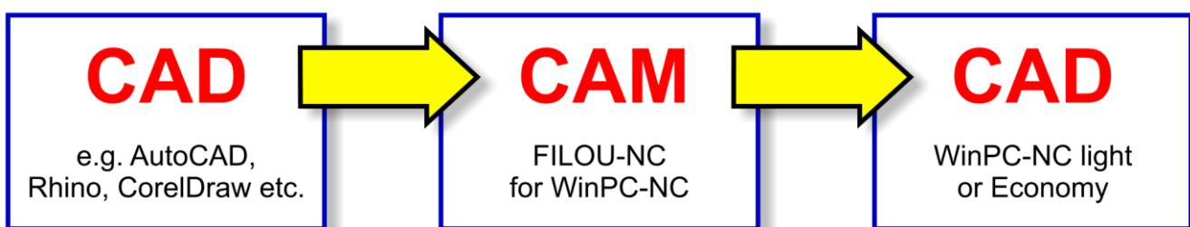
The workpiece to be manufactured is defined as geometry in a CAD program. CAD drawings are generally made at a scale of 1:1 and therefore they are perfectly suitable for creating NC-programs with a CAM program.
