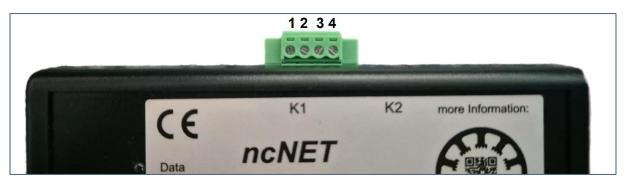
+12-36V: Connector K1 Pin 2 GND: Connector K1 Pin 4
