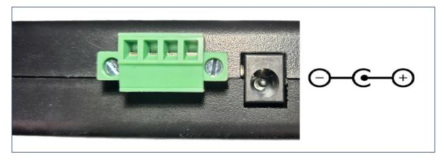
A coaxial power connector with 5.5/2.1mm or 5.5/2.5mm is required, positive pole inside.
