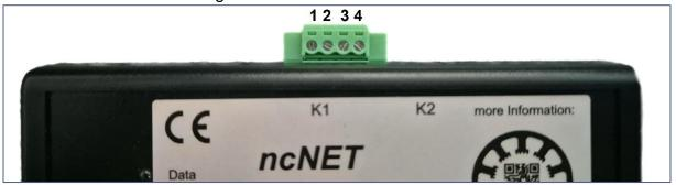
+5V: Connector K1 Pin 3 GND: Connector K1 Pin 4
