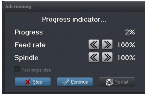
The Job running window with speed and spindle override
