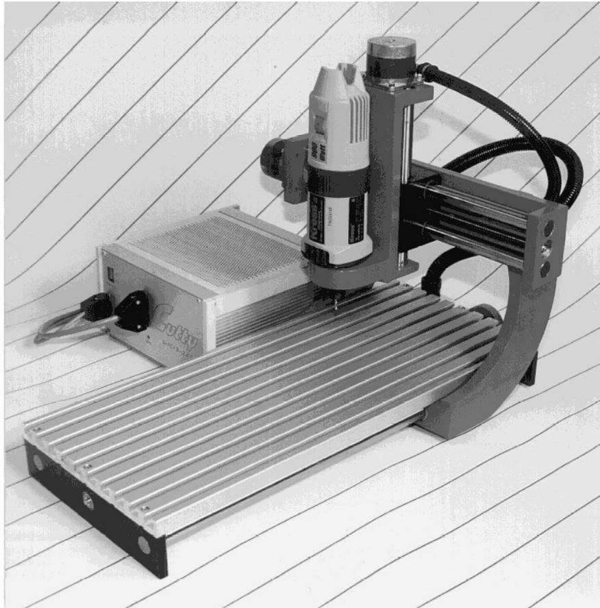
example for a 3 axis milling machine
